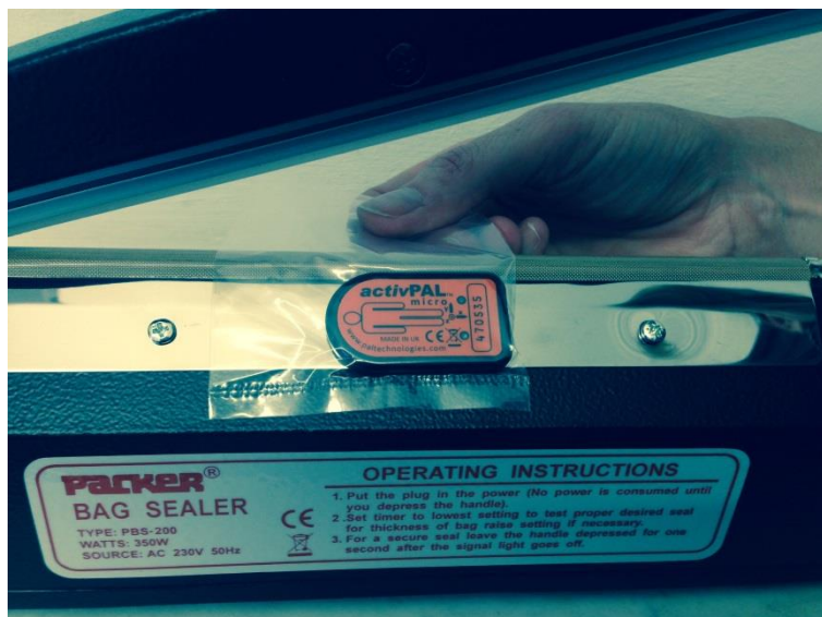
Figure 4: positioning the monitor in the sealing machine
