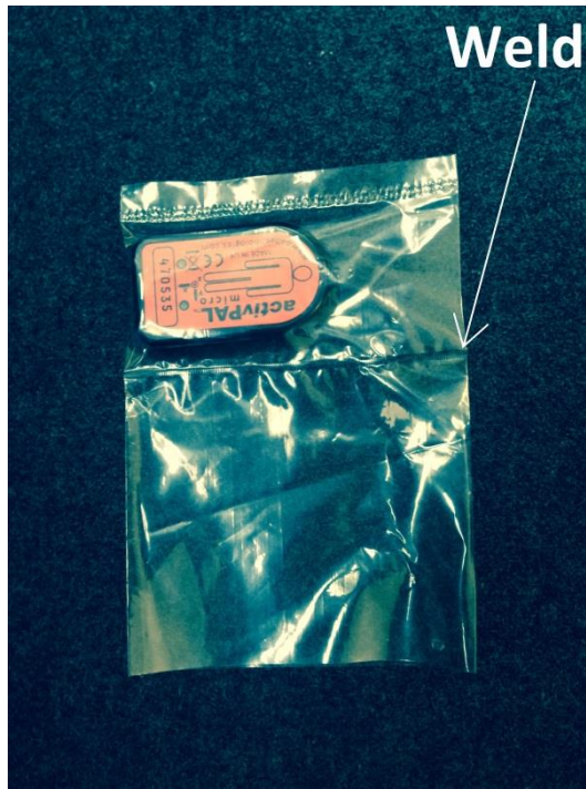
Figure 5: weld in bag
